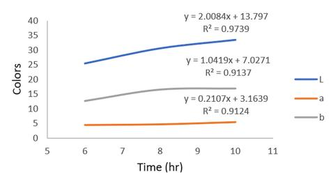
Figure 3. The relationship between the change in CIE-L\*a\*b values with drying time
